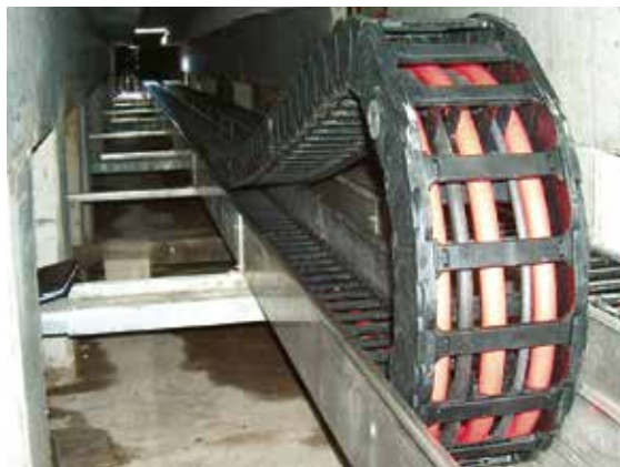
chainflex® CFCRANE for 500 m and more of travel. E-Chain®: igus® rol E-Chain®
