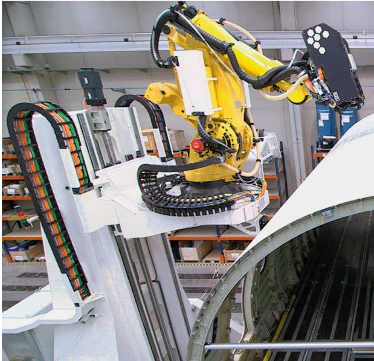
chainflex® servo cable in a vertical E-Chain®
