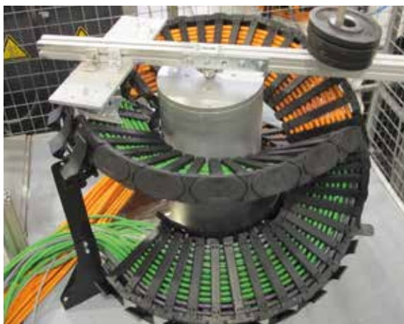
Rotary movement tests: Demanding chain applications with small radii
