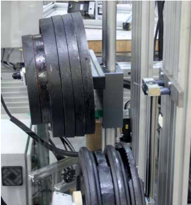
Test rig at the igus® lab to determine service life
