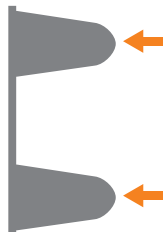
Rounded tooth profile, dryspin® geometry
