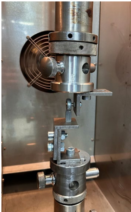
Tensile test in the temperature chamber
