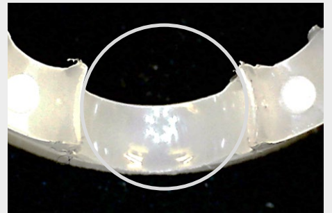
Unreinforced material, after the test
