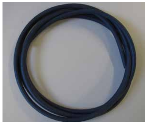
Result chainflex® TPE jacket: Cable after the test with 520,000 strokes
