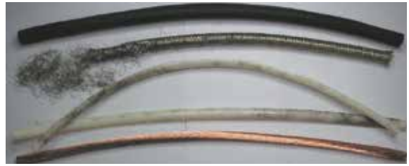
Picture 1: Damaged overall shield sample of the braid version after 250,000 torsional movements
