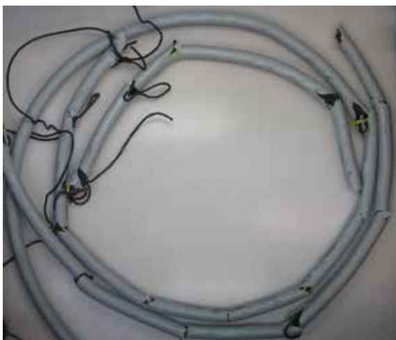
Result PUR jacket: Break already after 41,000 strokes
