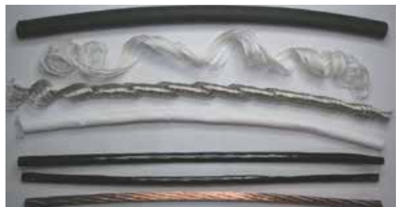
Picture 2: The CFROBOT shows absolutely no damage after more than 3 million movements
