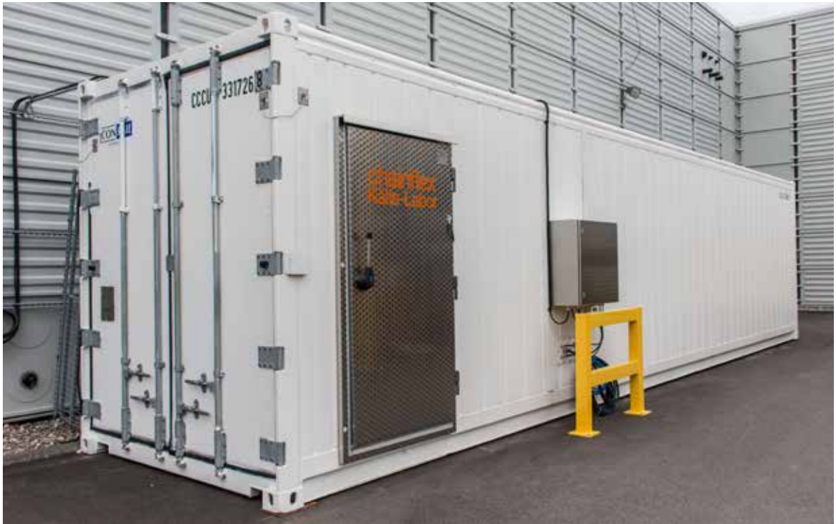
40-foot climatic container for cable tests in continuous motion at -40°F
