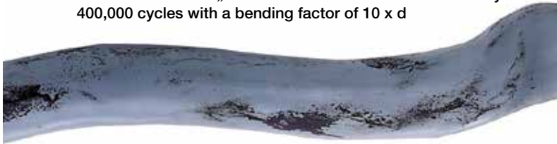
Picture 4: Shielded „chain-suitable“ control cable after only 400,000 cycles with a bending factor of 10 x d
