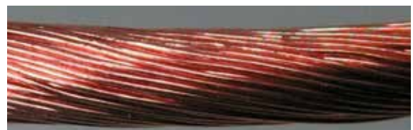
A close-up of the completely intact copper conductor. The inspection performed over the entire length shows that the conductor is still completely intact and does not have any individual wire breakages.
