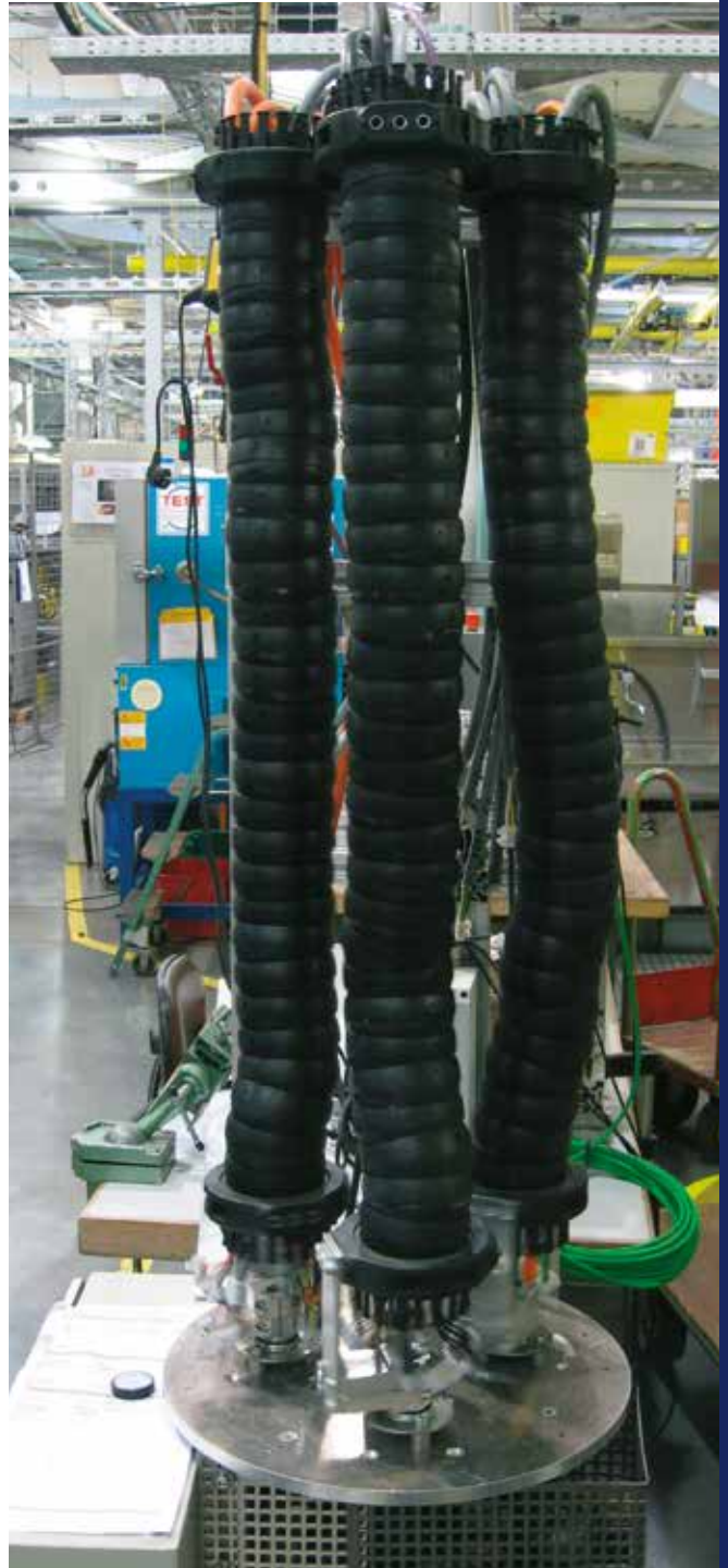
The „torsion test bench“ especially developed according to the igus® standard
