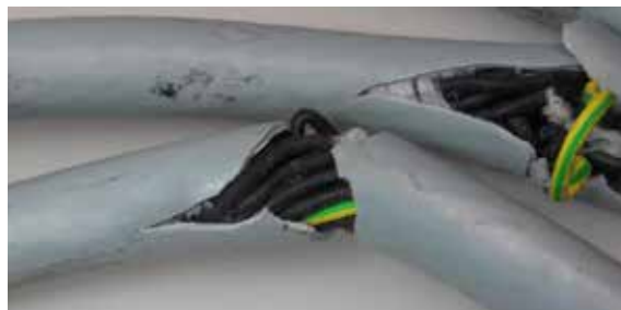
Jacket damage already after 41,000 strokes ...
