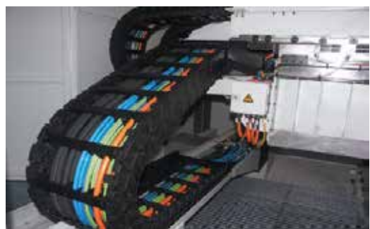
chainflex® measuring system cables in a double-spindle horizontal machining centre.
