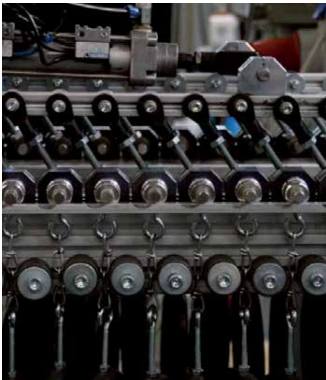
Picture 10: Wear test rig for testing the wear in pivoting movements at low loads
