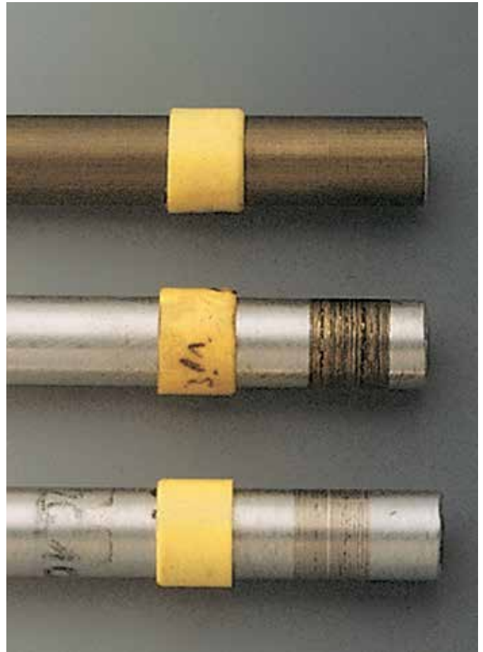
Picture 8: Wear experiments with aluminum shafts
