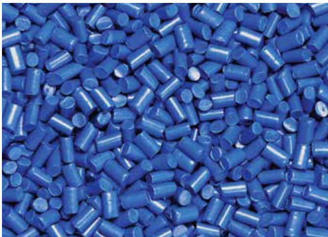
Picture 04: Polymer granulate; basis compound of the self-lubricating and predictable iglide® plain bearings
