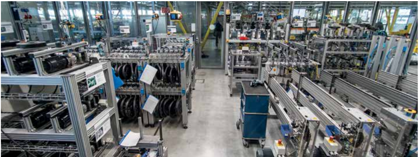
Picture 01: igus® test lab: 15,000 tribological tests (friction and wear) in 300 test set-ups in the industry's largest laboratory (40,900ft²). View inside bearing laboratory in Cologne
