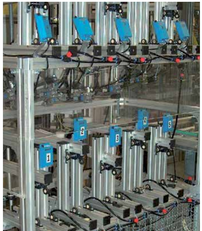
Picture 11: Wear test rig for testing the wear in pivoting movements at medium loads
