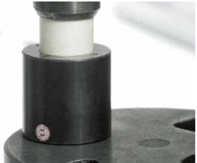
Picture 12: The bearing should be press-fit using a flat press
