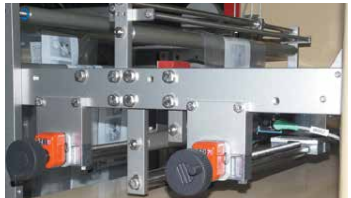
Train ticket detection The drylin® SLW linear actuators with position indicator and hand wheel adjusts the sensors which detect the edges of the train ticket and any print marks.
