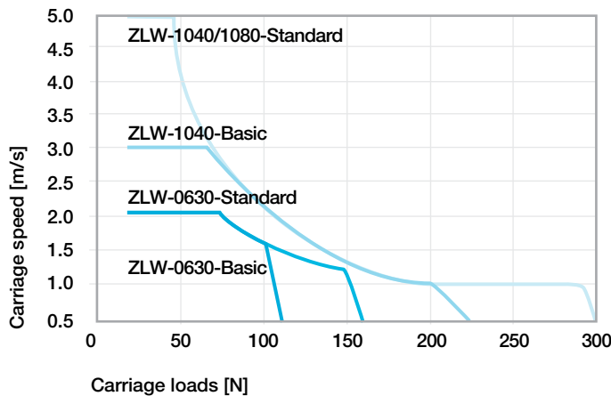
Diagram 11: Maximum load compared: ZLW-0630 and ZLW-1040/1080, 100% OT (On-time). The graph accounts for the sum of all forces active on the carriage.
