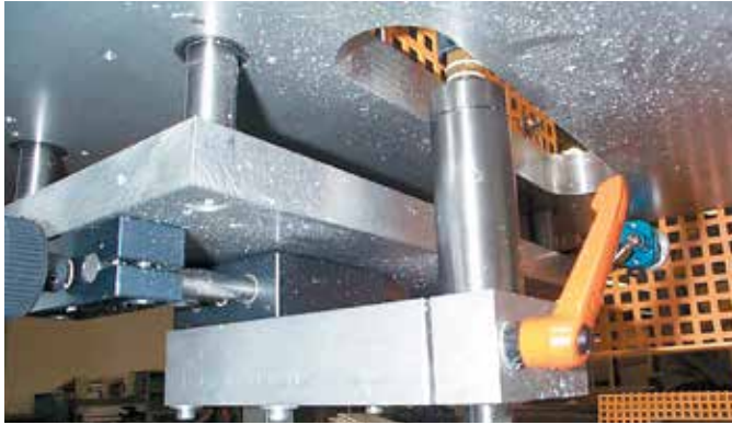
Milling head positioning drylin® lead screw tables work well in environments with metal shavings due to the lack of wet lubricants.
