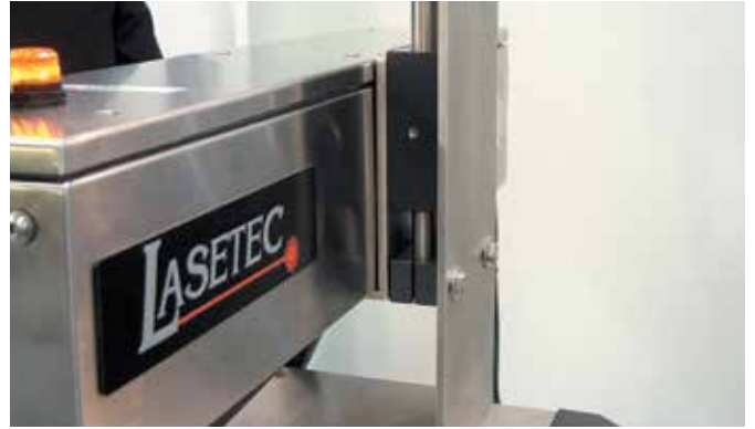
Height adjustment of coding device The drylin® linear actuators give variable and precise adjustment, free from any maintenance or lubrication. (Filtec Europe GmbH)
