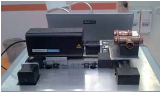
Adjustment of inspection camera drylin® ZLW toothed belt axis in an inspection camera adjustment for checking the position of sealing rings. (OLPE Jena GmbH)
