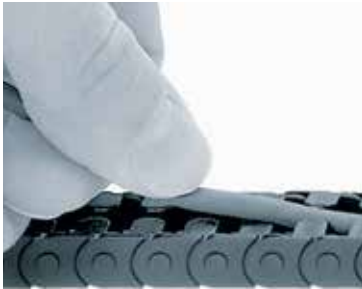
Just push the cables into the e-chain using your thumb
