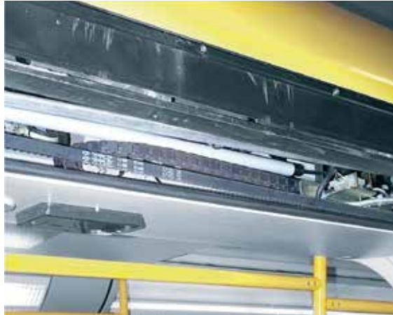
Long-travel applications up to 131 ft. (40 m) are possible - here: Series 10 in textile machine
