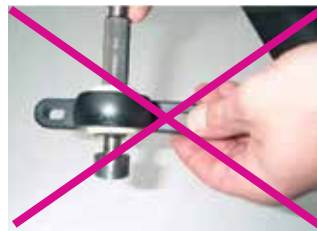
Inadequate test equipment; plug gauge too short
