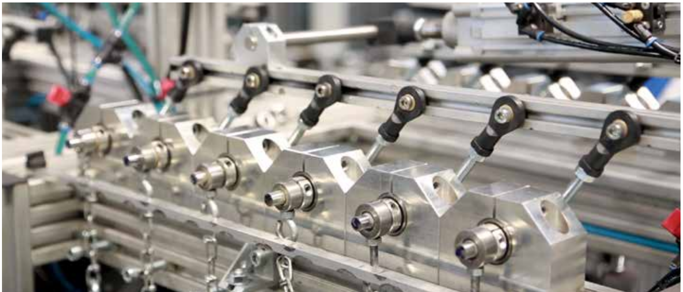
Picture 01: igus® test lab: More than 13,000 tribological tests (friction and wear) each year in 300 test rigs in the industry's largest laboratory (40,900ft²). View inside igubal® test rigs.
