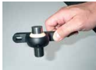
Tolerance test with plug gauge
